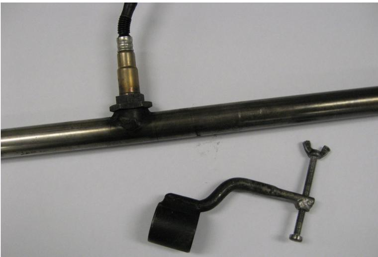
Sliding probe clamp and mounted sensor into main tube.
