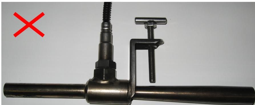
**Inaccurate, poorly designed probe (too small & fixed clamp position)!**
