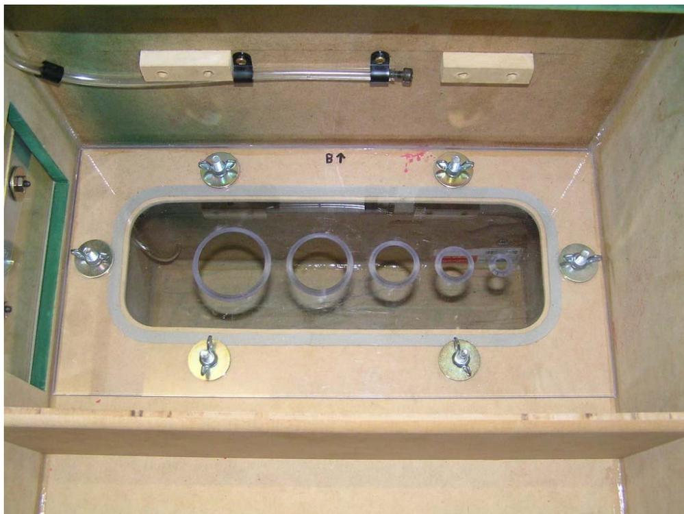
A view with the lid removed and the laminar flow grid in place above the orifice plate. The tube visible on the right is from the vertical manometer for measuring the test pressure.
