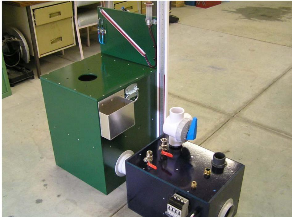
View with the lid removed. Visible is the orifice plate (no 'bungs' fitted in the photo) with captive bolts (bonded in) and wing nuts that allow the orifice plate to be turned over easily for blow testing of exhaust systems etc. Upper pressure sensing tube can be seen on the back wall, there is one below the orifice plate also, their ends are blocked and they have small holes along them (not visible). The wooden blocks on the back wall are what the laminar flow grid rests on.
