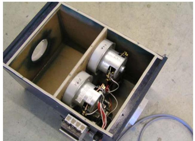
Made from MDF wood the main box is glued and screwed together. The lid is removable for maintenance and construction and screws on, it's sealed with foam 'weather strip' attached to the box lip.
