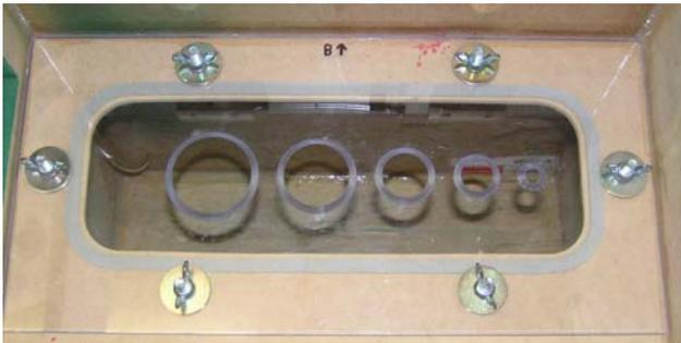
The edges must be angled steeply so that a sharp edge is formed and air does not 'follow' the taper and become turbulent. The direction of air flow when measuring must be with the air flow hitting the flat side (taper down stream). The whole plate is simply inverted for blow testing. This design behaves as a true 'sharp edge', this was confirmed by testing on a superflow SF-1020 bench at all reasonable pressures.
