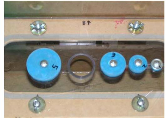
After experimenting unsuccessfully with machining and stamping of very thin gauge plates, the current orifice construction concept was reached. The holes are milled into a Perspex sheet and a steeply angled edge ensures that the edge is very sharp.
