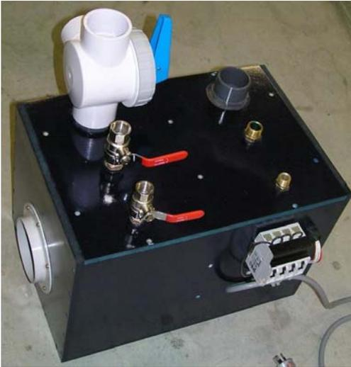
By keeping the airbox a separate unit it allows compact storage and easy modifications or upgrading if needed later. A simple PVC plumbing pipe slides into either end to attach to the main flowbench cabinet and the whole unit can be turned around to blow instead of suck.
