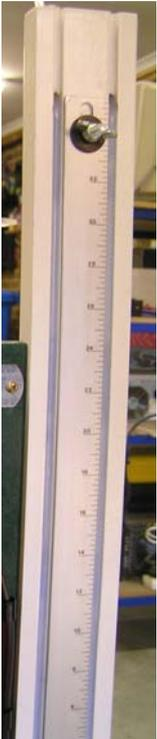
The vertical U-tube manometer on the side (large white strip in the photos) is for confirming the test pressure that's set by adjusting the air bleeds on the airbox.
