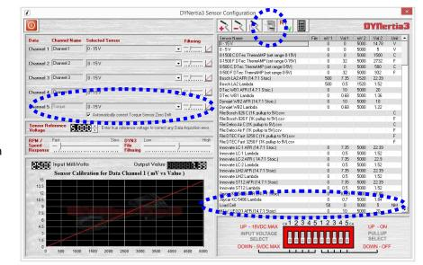
Note: This guided calibration procedure allows for automatic 'zeroing' of the load cell during use (it leaves a small 100mV offset voltage so DYNertia3 software can read a negative load if required). If you wish you can turn off, deselect "Automatically correct torque sensor for zero torque drift" in menu 'setup'/'sensor configuration'
