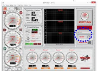
Due to limited screen space, with only a single monitor the data is displayed as shown to the Left. There are chart recorders and gauges for RPM, torque and power, whilst the 4 data channels are displayed on a second set of gauges with alarm limits.
