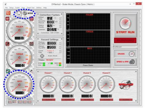
At this stage of setup the gauge will just be displaying dyno roller RPM, not engine RPM as no drive ratio has been specified
