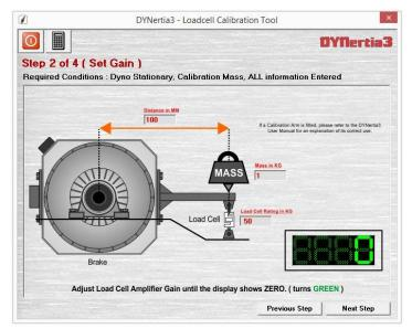
Step 2: requires applying a known weight and entering the data. Then the load cell amplifiers 'Span' (gain) is adjusted till the digits turn green.
