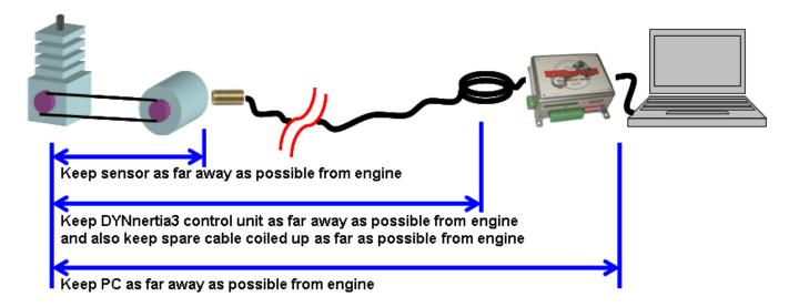
1) Mount the sensor unit at the furthest distance (<u>'every inch counts'!</u>) from the engine as possible. Route all cables as far as possible away from the engine (and any electric motors such as cooling fans) and keep the controller and PC at a distance. Coil any spare cable up neatly at the PC. Keep the sensors lead away from the USB lead or any other wiring.
