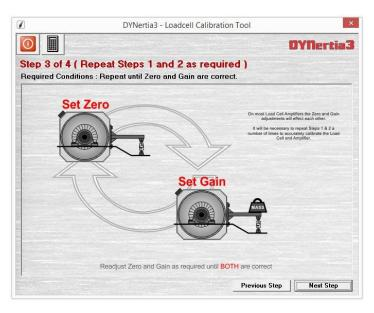
Step 3: asks to repeat the process to confirm. This is because with a load cell amplifier adjusting Span will effect Offset and vice versa.
