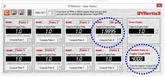
Drive vehicle until it's tacho matches the 'Engine Target RPM' in your test gear (4000 RPM in this example shown; alter this set point if RPM not suitable for your vehicle) then simply press a 'Compute Ratio' button, we will use "Compute Ratio 4" in this example to remind us we are testing in 4<sup>th</sup> gear. The calculated ratio will now appear in the box above the button (1.9895 in this example)
