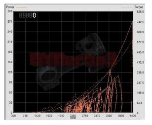
**NOT OK-** Crazy data due to electrical interference from the ignition system.
