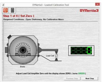
Adjust the amplifiers 'Offset' (zero or null) until the digits turn green as shown on the Right then press 'Next Step' button.
