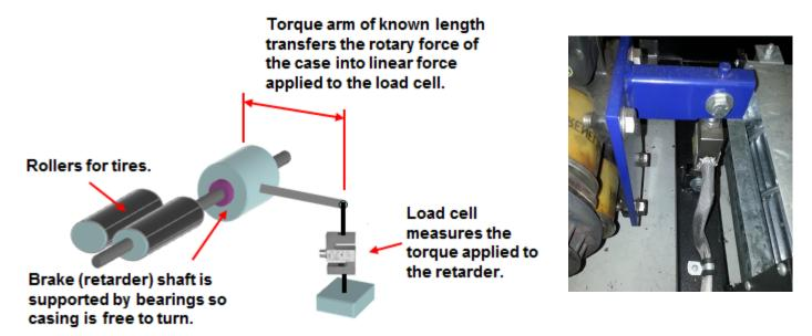
If we know the force (in Nm allowing for the length of 'torque arm') applied to the load cell and the RPM of the shaft we can calculate power by the metric formula  $Kw = (Nm \times RPM) / 9549$ , this will be power at the wheels. By using a chassis dyno we can have a very convenient and quick way of testing modifications, unfortunately the effect of drivetrain losses and tire losses do have an impact.
