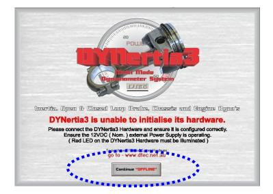
2. Plug the USB lead in, start DYNertia3 software, select the menu option "Setup" and then choose "Communication" and then press the "LINK" button to DYNertia3 to automatically configure the port interface. Then repeat for 'Weather Watch' if connected.
