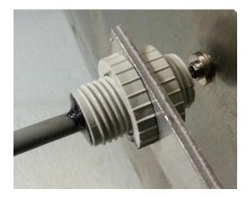
**dTip**- After the 'Linking' process (discussed later) the sensor operation can be checked via the button "DYNertia3 Sensor Test". The indicator and an audible noise can be used to confirm sensor operation during <u>slow</u> rotation. The indicator lamp/noise triggers for a short time as the magnet approaches the sensor (only on approach).
