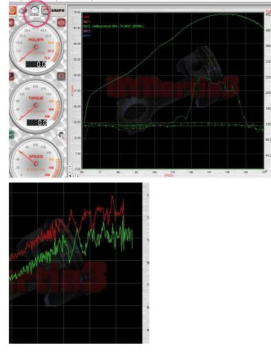
**NOT OK**- Power traces getting very erratic as speed rises. Mechanical issue creating variations in shaft speed (vibrations or 'snatch'). Greater filtering will help somewhat but not a fix.
