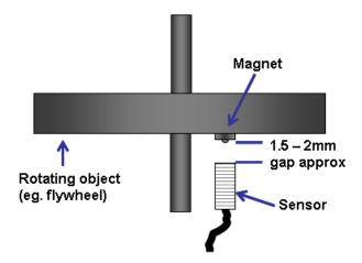
The sensor face <u>must be positioned 1.5 - 2mm</u> from the magnets <u>South Pole</u> (or the head of the screw if one is used to secure magnet).
