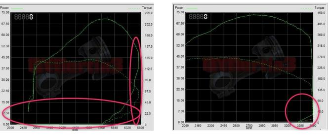
**NOT OK-** Both these traces are running back under themselves at the test end. The trace should <u>not</u> run back under itself or you effectively end up with 2 power readings for every RPM point and this is confusing to calculations we run.
