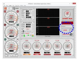
Due to limited screen space, with only a single monitor the data is displayed as shown to the Left. There are chart recorders and gauges for RPM, whilst the 4 data channels are displayed on a second set of gauges with alarm limits.
