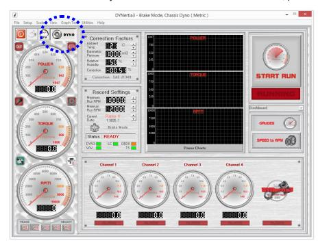
Note: The Row of gauges (input channel data) shown along the bottom of the screen are visible with a single monitor. With duel monitors this data is displayed on the second monitor instead and replaced with the test 'comments' field (also found in 'View' menu).
