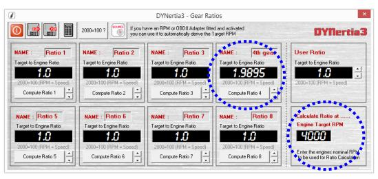
Ride the bike until the bikes tacho matches the 'Engine Target RPM' in your test gear (4000 RPM in this example shown; alter this set point if RPM not suitable for your vehicle) then simply press a 'Compute Ratio' button, we will use "Compute Ratio 4" in this example to remind us we are testing in 4<sup>th</sup> gear. The calculated ratio will now appear in the box above the button (1.9895 in this example)
