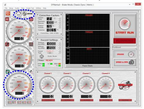
At this stage of setup the gauge will just be displaying dyno shaft RPM, not engine RPM as no drive ratio has been specified
