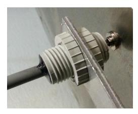
**eTip-** After the 'Linking' process (discussed later) the sensor operation can be checked via the button "DYNertia3 Sensor Test". The indicator and an audible noise can be used to confirm sensor operation during <u>slow</u> rotation. The indicator lamp/noise triggers for a short time as the magnet approaches the sensor (only on approach).
