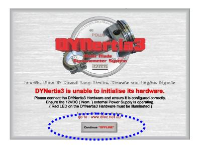
Plug the USB lead in, start DYNertia3 software, select the menu option "Setup" and then choose "Communication" and then press the "LINK" button to DYNertia3 to automatically configure the port interface. Then repeat for 'Weather Watch' if connected.
