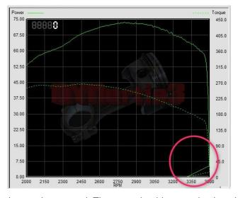
**NOT OK**- Both these traces are running back under themselves at the test end. The trace should <u>not</u> run back under itself or you effectively end up with 2 power readings for every RPM point and this is confusing to calculations we run.
