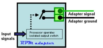
The DTec 'RPM adapter' is designed to turn signals from many different sources into compatible signals for connecting to digital devices, such as DYNertia's 'RPM Adapter' input (DYNertia3 uses this input to provide an optional second RPM source).
