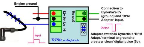
**NOTE:** If you are using an inductive clamp (e.g. from a timing light) you will find that only one wire will generally need connecting to the Lo terminal i.e. the coil in the clamp is left with one end not connected.
