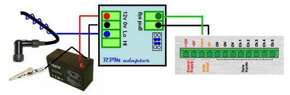
**NOTE:** As shown, you can use a separate power supply source for 'RPM adapter' unit if required to avoid interference issues by keeping 'RPM adapter' completely isolated from other equipment! Ground for engine is optional (see below).
