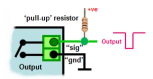
RPM adapter does not send out a voltage pulse, it is a switching device. If not connected to DYNertia3 you must connect a ground and a 'pull-up' resistor as shown, then you can measure a pulse output on the "sig" terminal as the switch opens and closes. The switching current should be limited to < 40mA, we suggest a 10K ohm pull-up resistor.
