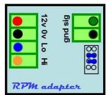
Output terminals. These are bridged together to create a switch that stays closed for the time set by the 'mode setting'. They are fully isolated from the rest of the circuitry for protection and freedom of use.
